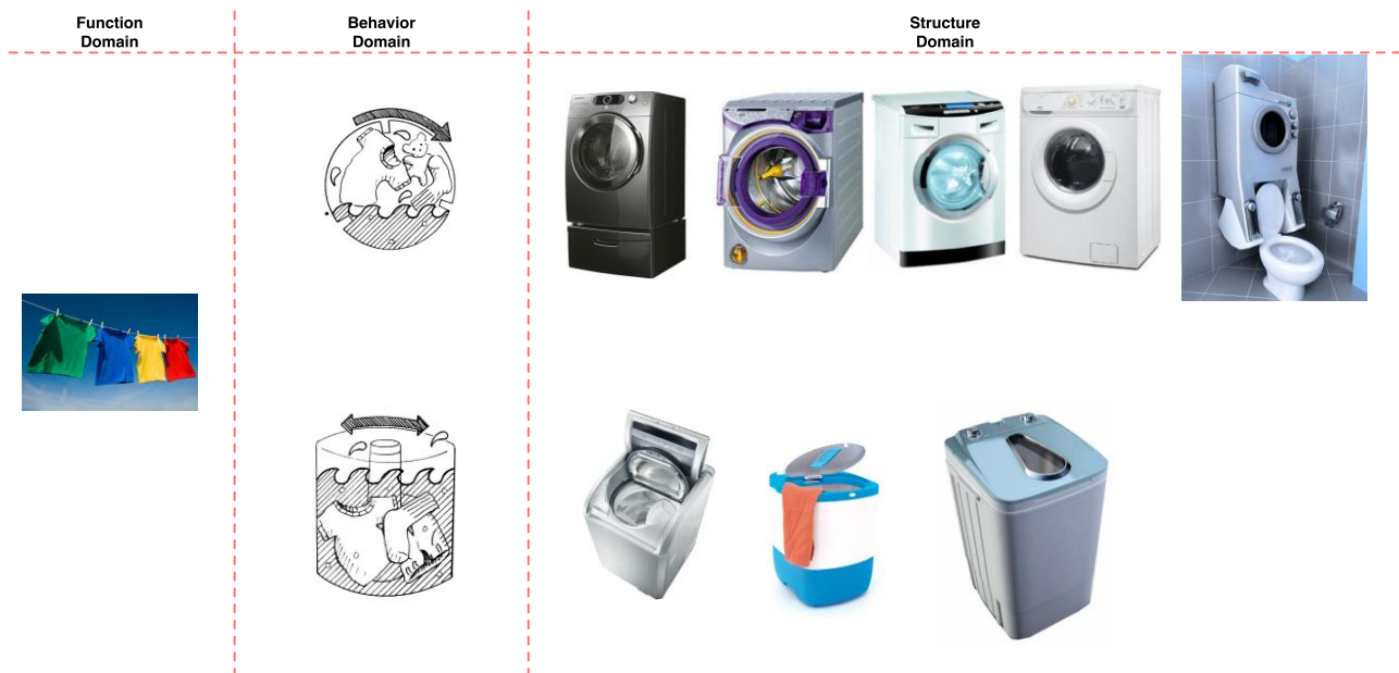
Figure 66: The organization of different solution according to the pertaining domain. All the presented solutions accomplish the function of cleaning clothes (left image). The washing machine to produce such a results can be characterized by different behaviours. Among them there are the ones using a drum whose axis could be horizontal (on the top of the figure) or vertical (on the bottom of the figure). Alternative structures are presented on the same line.
